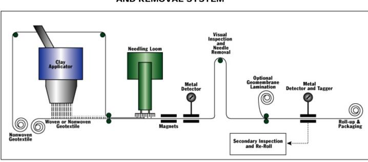
SCHEMATIC OF NEEDLE DETECTION AND REMOVAL SYSTEM
