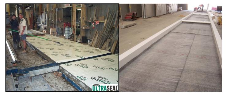
VOLTEX or ULTRASEAL can be either placed on top of the still wet Panel or placed directly on to the Panel Table and Mould depending on the desired internal Panel finish.
