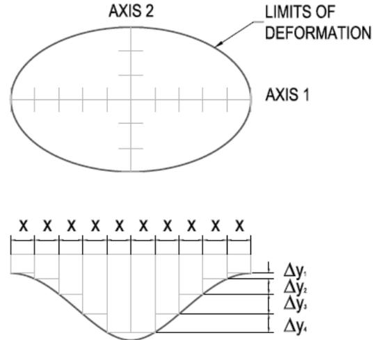
**Figure 2. Geomembrane Deformation Measurement Method**
