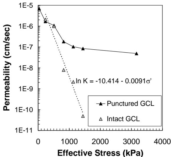
**Figure 4. GCL Permeability With Copper PLS**
