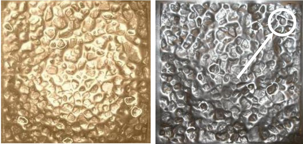
Figure 1. Comparison of 60-mil (1.5 mm) LLDPE Geomembrane tested in contact with 1/2" to 1" (12 to 25 mm) rock at 585 psi (4033 kPa) for 48 hours, both with (left) and without (right) underlying GCL.
