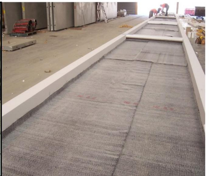
VOLTEX or ULTRASEAL can be either placed on top of the still wet Panel or placed directly on to the Panel Table and Mould depending on the desired internal Panel finish.
