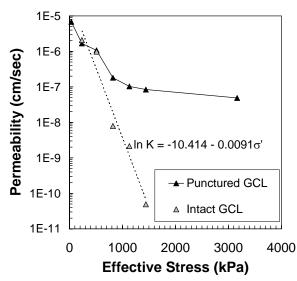
Figure 4. GCL Permeability With Copper PLS
