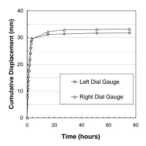
**Figure 1. Geomembrane Deformation Readings**
