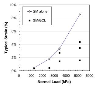
Figure 3. Geomembrane Strain vs. Normal Stress
